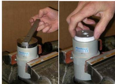
First screw cap (air outlet), remove piston and spring then disassemble socket.
